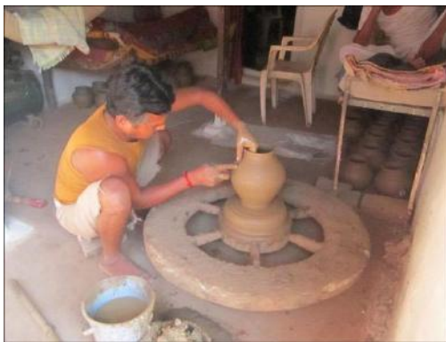
Fig. 3b: Iron tool (scraper type) used for scraping off the unwanted clay
